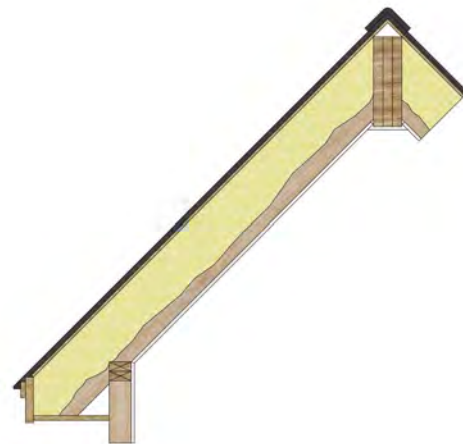
Figure 5. Insulated Rafter Assembly
