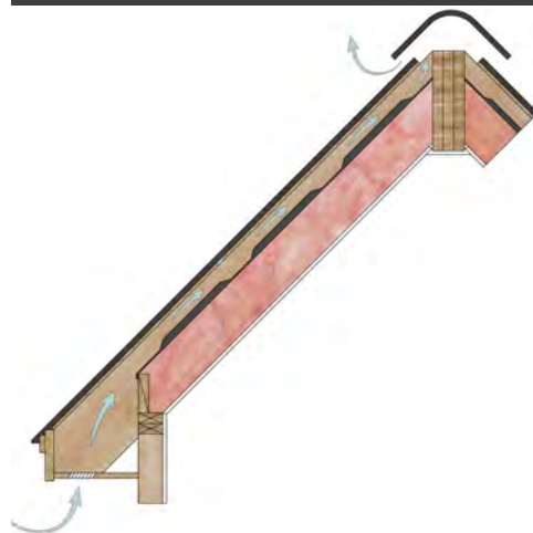
Figure 2. Vented Roof Assembly
